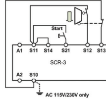
Fig. 4: Two-channel sliding guard monitoring with short circuit and earth fault monitoring. (category 4, up to PL e)
