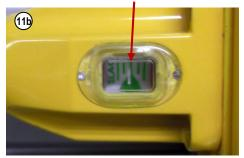
11c. For long rope spans >50m. it is advisable to balance the system by making turns to the Left and Right Tensioner/Grippers in turn whilst at the same time checking the rope tension setting in each of the switch viewing windows.
